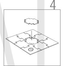
Place the center part. It has to be the last piece to be assembled.
