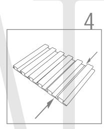
You can also adjust the amount of absorption by cutting one or more stripes, tuning the sound as desired.
