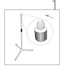
Start tightening the nut on the tripod.
