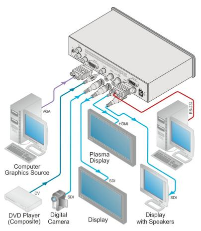
Figure 2: Connecting the VP-460 Video Scaler
