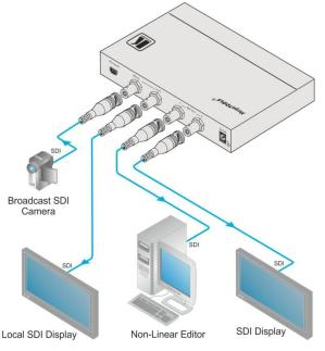
Figure 2: Connecting the VP-470 SD / 3G HD-SDI Scaler
