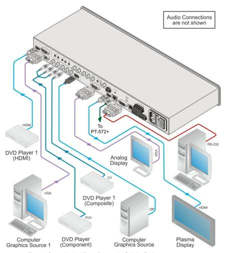
Figure 4: Connecting the VP-770 Presentation Switcher/Scaler
