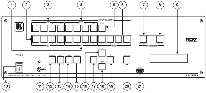
Figure 1: VP-725N Presentation Switcher / Scaler Front Panel
