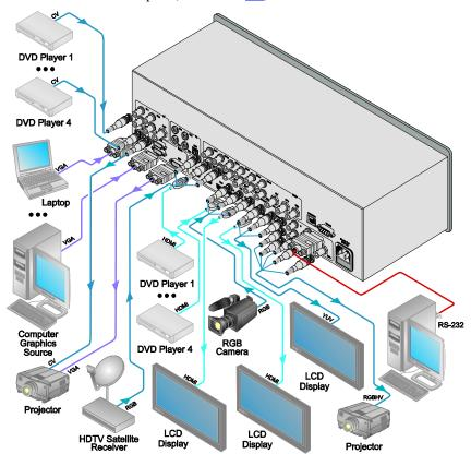
Figure 3: Connecting the VP-725N Presentation Switcher / Scaler
