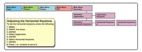
Figure 20: Example of how to use the LCD Display
