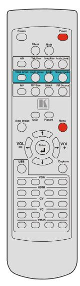
Table 17: Infrared Remote Control Transmitter Functions
