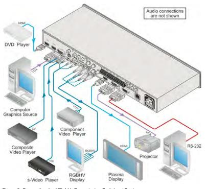
Figure 3: Connecting the VP-441 Presenta ion Switcher / Scaler
