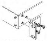
2. Place the ears of the machine against the rack rails, and insert the proper screws (not provided) through each of the four holes in the rack ears.
