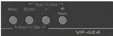
If you cannot see the display after factory reset, use the front panel buttons to set the correct resolution (as indicated on the panel):
