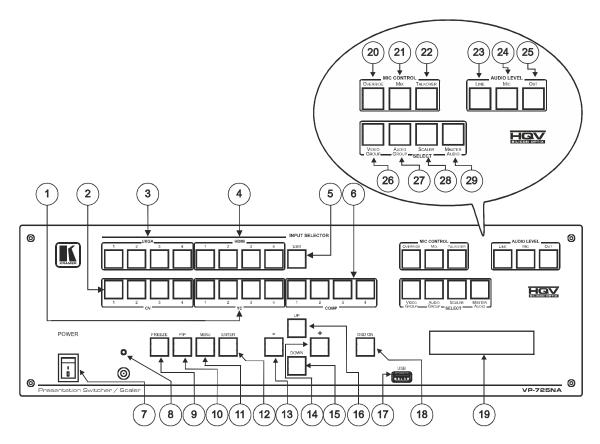
Figure 1: VP-725NA Presentation Switcher/Scaler Front Panel
