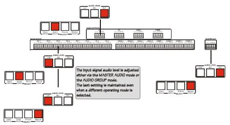
Figure 12: Adjusting the Audio Input and Audio Output Levels
