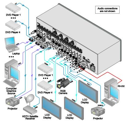
Figure 3: Connecting to the VP-725NA Presentation Switcher/Scaler
