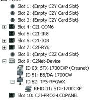
Double-click the STX-1700 (Cresnet) icon in the upper pane to open the "Device Settings" window. This window displays STX-1700 (Cresnet) device information. Select the *Net ID* tab to change the touchpanel Net ID, as shown in the following graphic.
