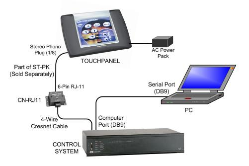
**NOTE:** If the control system in use has a 4-pin network connector rather than a modular (RJ-11-type) NET connector, use an ST-CBL interface cable (sold separately).
