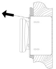
2. As shown below, insert a long-reach screwdriver into the access hole at a downward angle (approximately 10°) until the tip of the screwdriver contacts the manual unlatch tab.
