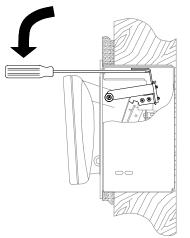
4. Refer to the diagram below. By hand, undock the touchpanel by pulling the upper edge of the touchpanel outward and remove the touchpanel.
