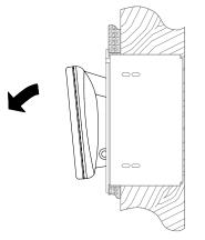
5. Refer to the diagram below. Re-install the access hole plug into the access hole.
