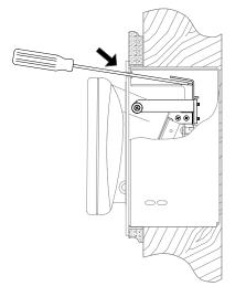
3. As shown below, lower the handle of the screwdriver until the touchpanel unlatches (handle of screwdriver will be approximately level and touchpanel will snap outward slightly).
