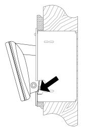
2. Refer to the diagram below. Make sure that the STX-1700CXPW is **squarely seated** in DA-1700CW, and press upper edge of touchpanel inward to dock the touchpanel. The touchpanel will snap into position.
