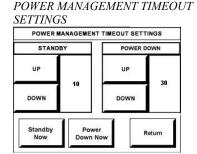
POWER DOWN timeout turns off all power when the touchpanel is inactive for the specified time. When the touchpanel is activated, either the first page of the project appears or the last screen to be displayed reappears, depending on the setting of the Power Up On Last Page option on the Startup Preference screen. The specified time is displayed in minutes. The default POWER DOWN timeout is 30 minutes.
