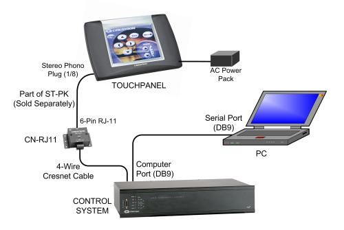
**NOTE:** If the control system in use has a 4-pin network connector rather than a modular (RJ-11 type) NET connector, use a ST-CBL (sold separately).
