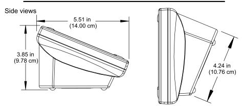
Four rubber feet on the underside of the unit are for stability and to prevent slippage on flat surfaces.
