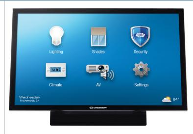
touch screen control system. For instance, using a DM switcher such as the DM-MD8X8<sup>[1]</sup>, multiple TSD-2020 touch screens can be connected to a single DGE-2, providing a simple, cost-effective way for multiple participants to view and control the same graphical interface. DigitalMedia also provides a versatile means for distributing touch screen content to additional display devices and sound systems to serve a larger audience.
