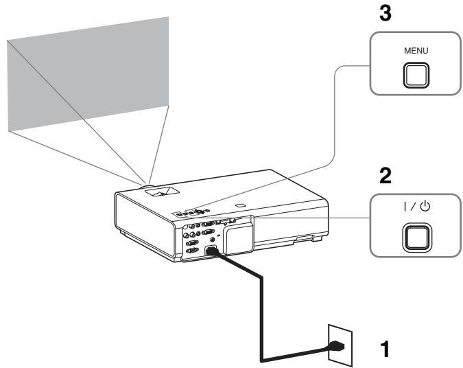
1 Plug in the AC power cord into a wall outlet.
