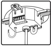
5. Connect Signal wire into terminal block
