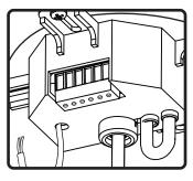
6. RS31-EZ-T wiring: Connect the negative signal wire to "com" and the positive signal wire to the desired power tap as indicated.
