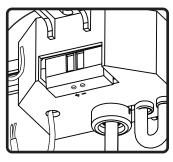
7. RS31-EZ wiring: Connect the negative signal wire to the (-) negative input and the positive to the positive (+) input.
