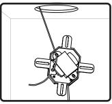
2. Feed signal wire from ceiling 3. Where needed, connect through the mounting plate via wire opening.
