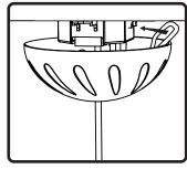
10. Excess wire can be hidden inside of cover plate by wrapping excess wire clockwise and into gap between plate and surface
