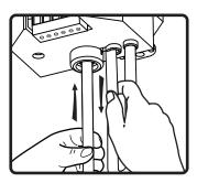
8. Set speaker height by adjusting speaker wire. Push wire through the central hole while pulling on the center slack line to shorten the speaker hanging height. Reverse to lengthen.
