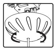
9. Move cover plate up speaker wire, begin to thread cover plate into mounting plate, leaving half an inch between cover plate and mounting surface.
